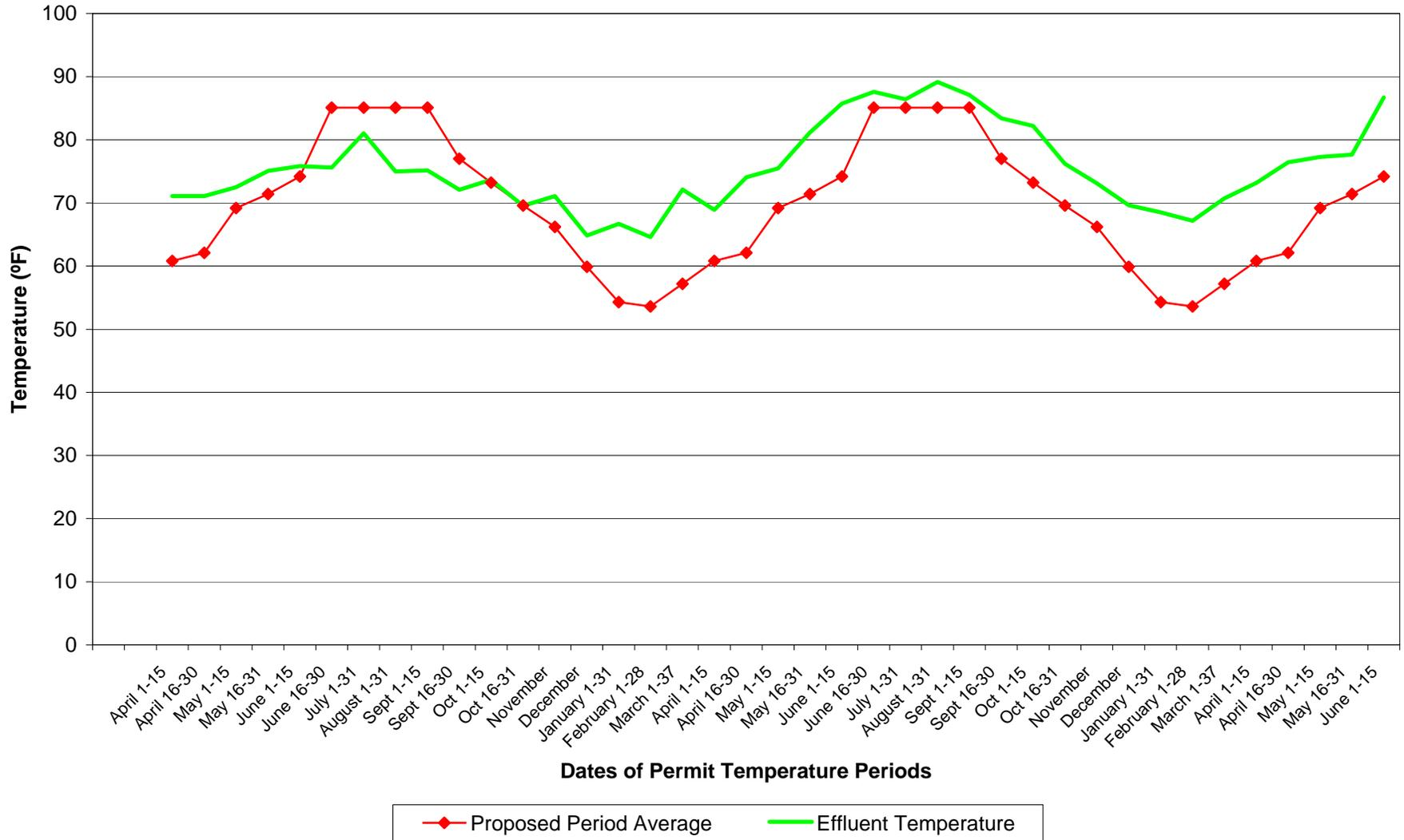
Figure 4. Cooling Required To Attain Discharge Limits
